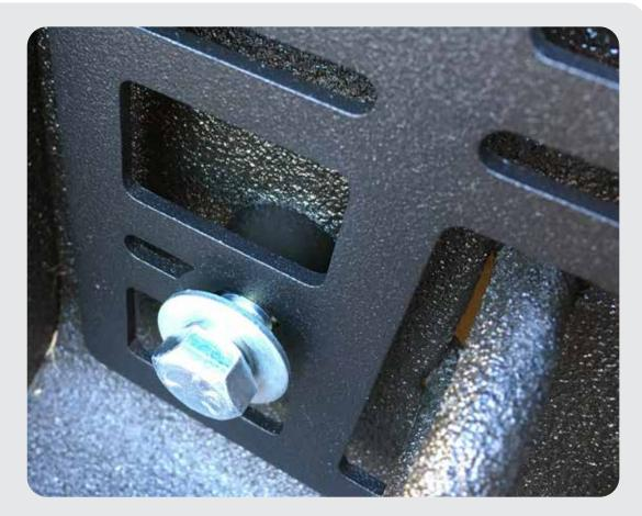
That finalizes your installation. The Upper Panel will work on the Driver's side or Passenger's side. If you have the lower panel it will bolt on to the upper panel in either direction and work for either side of the bed. There is a full lower MOLLE panel that works for either side of the bed. If you have the factoy bed outlet, there is a lower MOLLE panel available with a cut out to retain use of the bed outlet.
