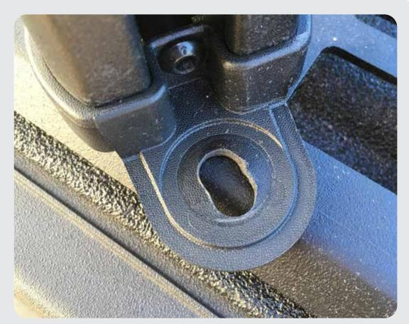
You will also need to cut off the plastic pin located on the back of the Trail Rail on the tailgate end of the bar. This is the end that has the plastic piece that you slot in the step above. Cutting this plastic pin allows the Bed Side MOLLE Panel to slide into place correctly. Be sure NOT to cut the plastic pin on the cab end of the rail, it helps with installation as it helps hold the end of the rail in place while placing the screws for installation.
