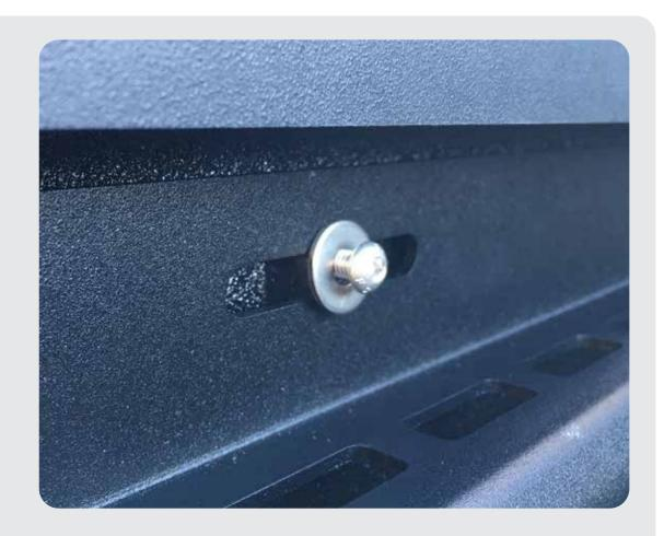
If using the Trail Rails, use the existing rail screws with the panel mounted under the rail. Keep all screws a bit loose until you align the lower corner bolt hole.
