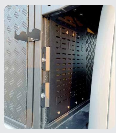
Installing the RotoPaX Mount: Using the pre-installed Rivnuts, add thread lock to all screws. Install the lower bracket first (1). Next, install the upper bracket (2) but keep the screws loose enough to adjust the height of the upper bracket so it is snug with your RotoPaX installed. There is a supplied plate to use with a pad lock. (Pad lock not included)
